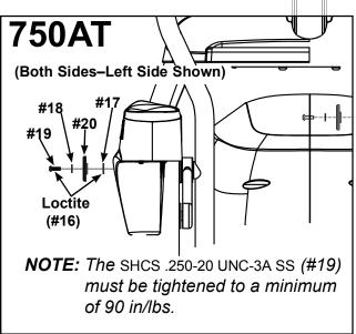
8. Verify the SHCS .250-20 UNC-3A SS (#19) are tightened to a minimum of 90 in/lbs.
