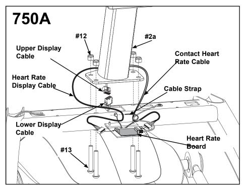
2. Plug the heart rate display cable (threaded through console mount in step 8C) into the heart rate board. Ensure cable connectors are securely fastened. Tighten cable strap. Refer to above the diagram.
