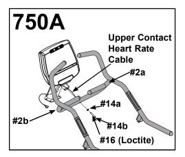
4. Attach the console assembly (#2a) to the handrail assembly (#2b); using a 7/32" Allen wrench, secure with one saddle washer .390 ID x .750 OD x 6 (#14a) and one BHSCS .375-16 x 2.25 SS (#14b). Refer to the above diagram.
