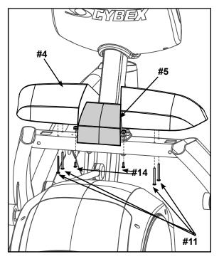
3. Using a Phillips screwdriver, securely fasten the four tap SC 10-12 x 2.00 Type A PN HD PHIL (#11).
