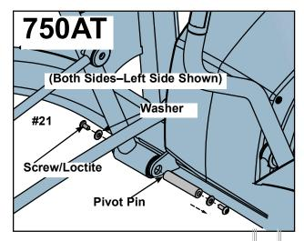
2. Apply loctite (#16) to threads inside the arm and both screws removed in step 2 of **Remove left** and right handle assembly.
